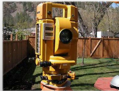
Topcon ET-1 Total Station. Manufacture Date: 1985. Dates of Use: 1980's. Source: NOAA
