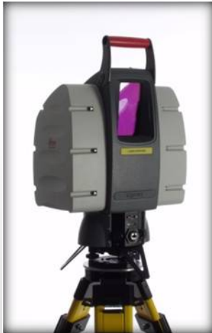
Ground-based static laser scanner mounted on a tripod. Source: Nobles Consulting Group
