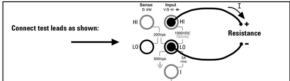
To null-out the test lead resistance:
