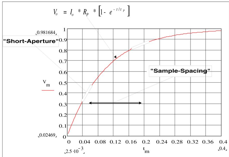
Capacitance is calculated by measuring the change in voltage (DV) that occurs over a “short aperture” time, (Dt). This measurement is repeated at two different times during the exponential rise that occurs. An algorithm takes the data from these four points, and by linearizing that exponential rise over these “short apertures”, accurately calculates the capacitance value.
