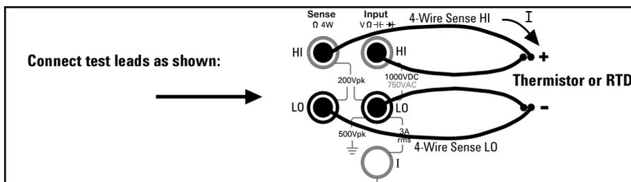
*All 4-wire temperature measurements are made with auto-zero on.*
