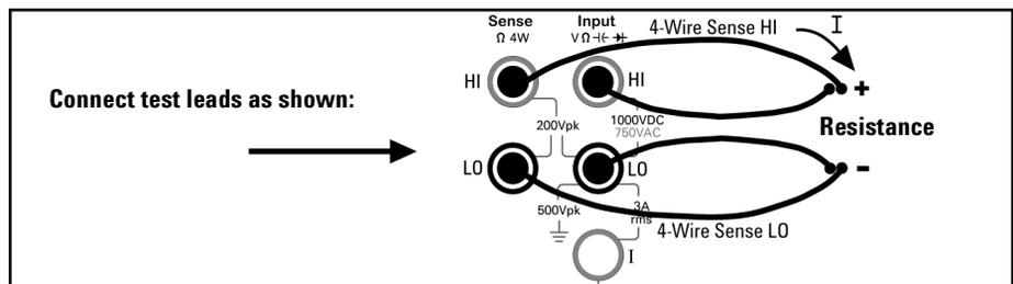
All 4-wire resistance measurements are made with auto-zero on.
