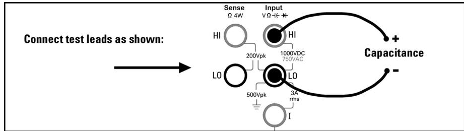
*To null-out the test lead capacitance:*
