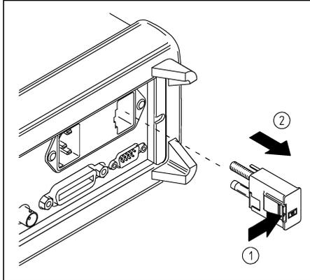
2 Remove line-voltage selector from fuse holder assembly.
